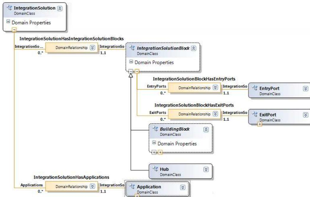
Fig. 2. Part of Guaraná’s metamodel represented in MS/DSL Tools.
